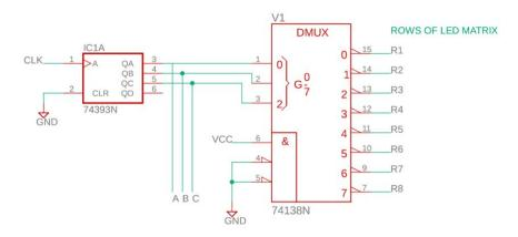
The clock output is given to counter which counts from 7 to 0 (down ripple counter). The counter is a 4 bit counter but we made use of only 3 output pins hence using it as 3 bit counter. Its output is connected to the inverting decoder as shown in the schematic. Reset pins of both IC's are connected to the ground or Vcc according to
